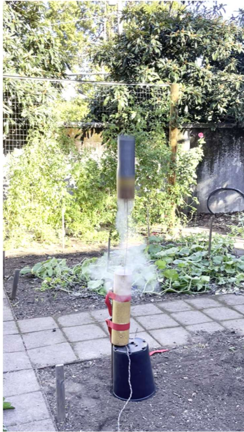
Figure 9-2 Energetic deployment for the large deployment fixture using 0.3 gm black powder from a frame of a video of the test
