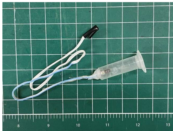
Figure 7-2 Black Powder charge canister
