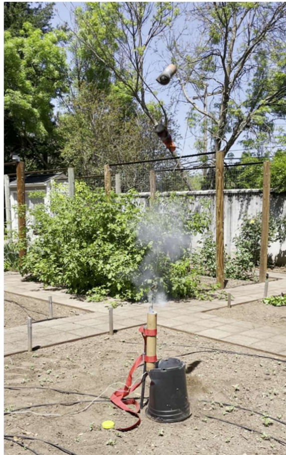
Figure 9-4 Energetic deployment of TR-1 fixture with 1.3 gm of black powder
