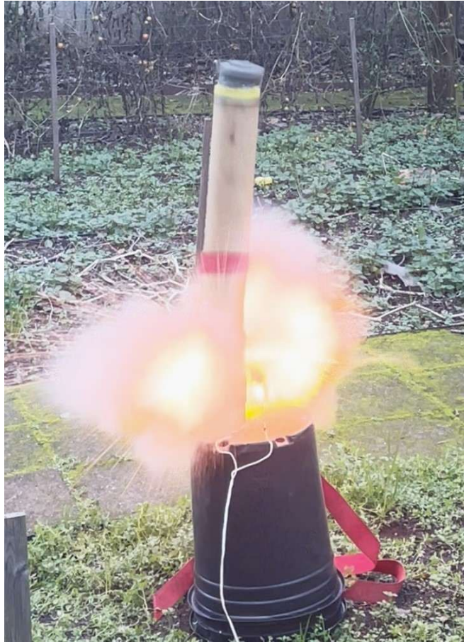
Figure 15-1 Failure of the airframe at 4.0 gm of black powder
