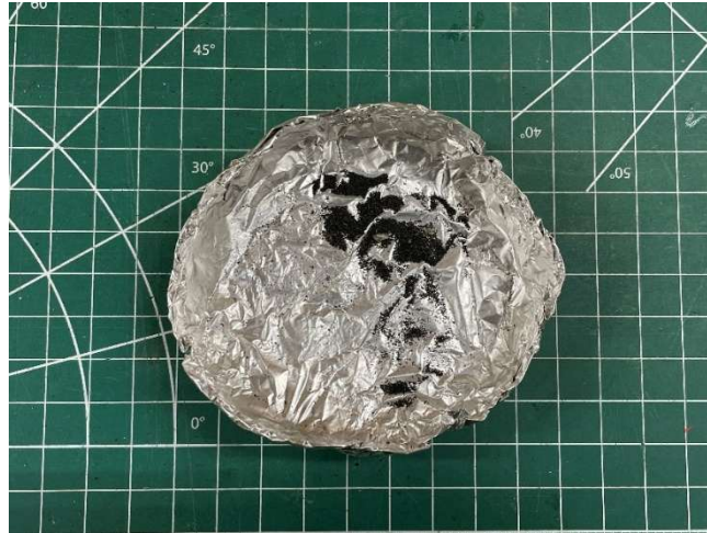
Figure 11-4 Unburned black powder residue left in bottom of test chamber
