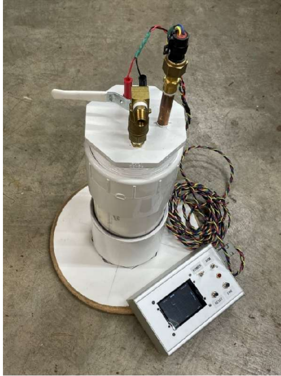
Figure 7-1 Black powder test chamber
