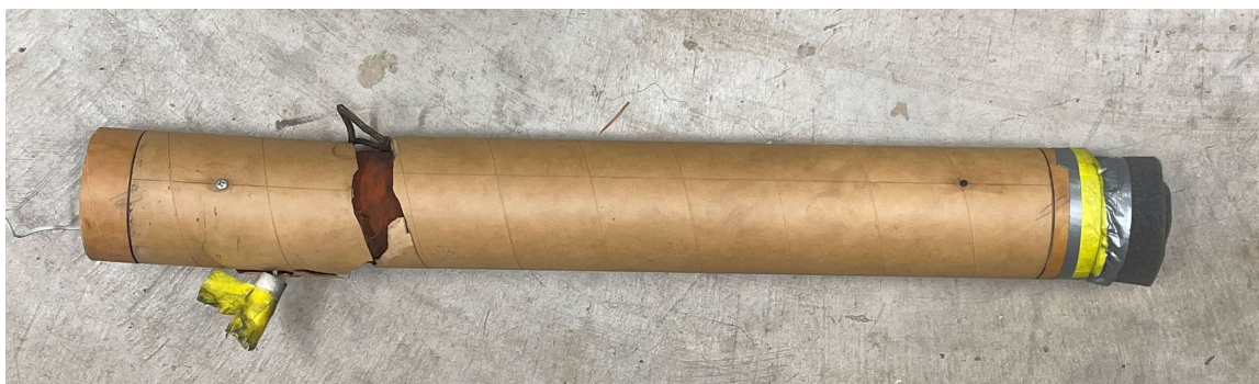
Figure 15-2 Damage to airframe from 4.0 gm of black powder showing the shear pins and nosecone still intact and the charge canister outside the tube
