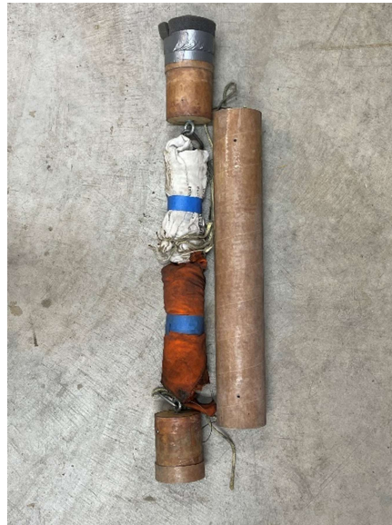
Figure 9-5 VTS-1 and the deployment test fixture with two parachutes
