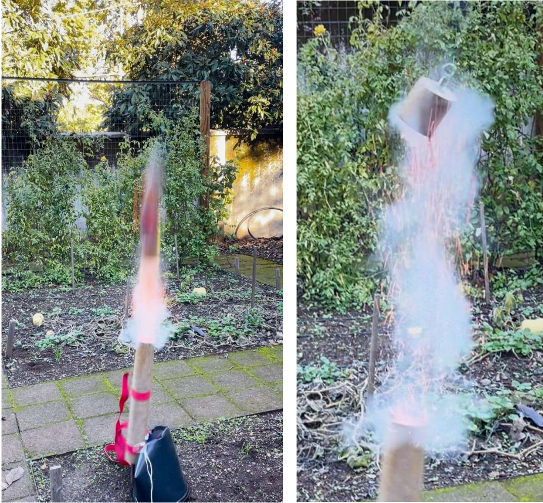
Figure 13-3 Two frames of the 1.0 gm piston deployment
