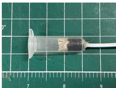
Figure 11-6 0.5 gm of black powder in a centrifuge canister
